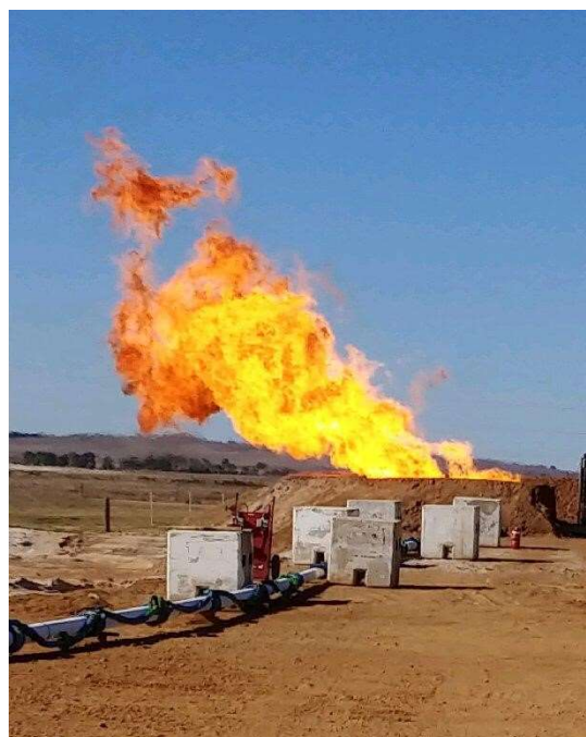
Figure 1 - flaring gas at surface on during D Sand testing
